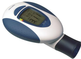
Figura 3: Aparelho Peak Flow Meter for Spirometry (Microlife PF 300) .
