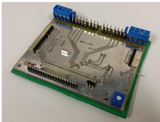
Figura 63 – Hardware principal de controle do eSurg-Arm
