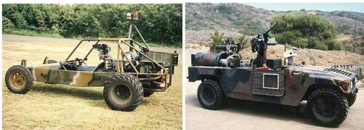
Figura 3 – TeleOperated Dune Buggy (SPAWAR Systems Center) e TeleOperated Vehicle (SPAWAR Systems Center).
