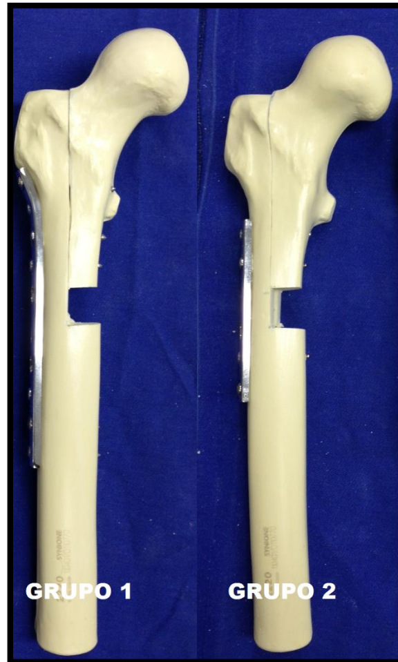
Figure 7 -bone models of proximal femur after "L" osteotomy divided into two groups according to the setting.
