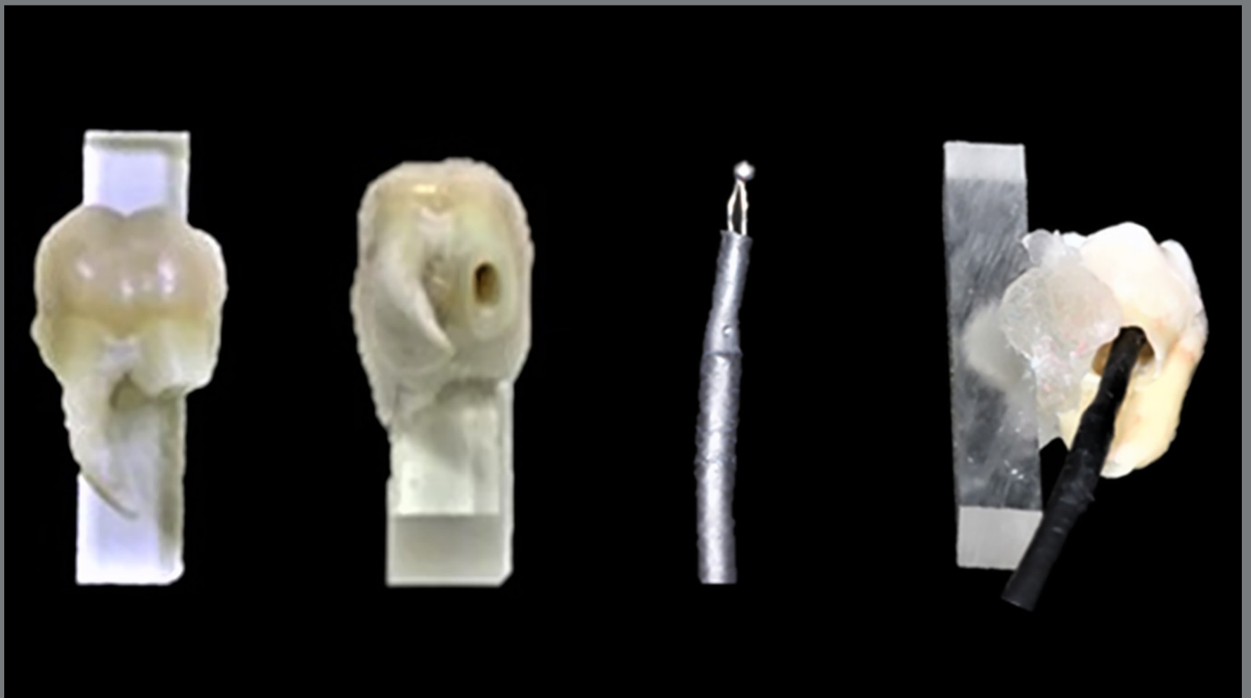
Figure 1: Specimen and thermocouple device inserted in the tooth root.
