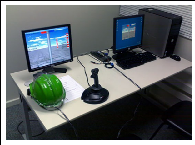
Figure 1. Physical components of the control station. The equipment includes an HWD, head-tracker, and joystick. HWD: head-worn display.
