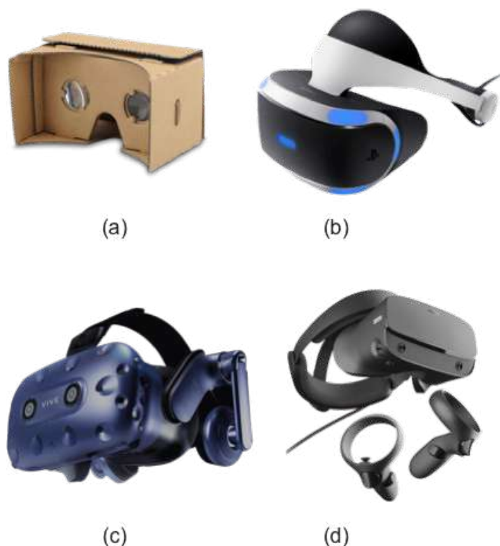
Figure 2 – VR devices. (a) Google Cardboard, (b) Sony VR, (c) HTC Vive and (d) Oculus Rift
