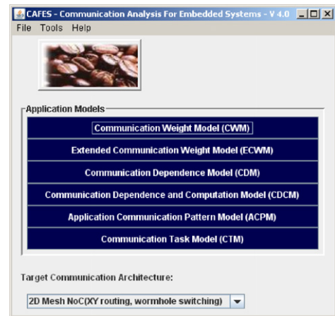
Fig. 3. CAFES initial screen, displaying the choice of application models and target communication architecture.
