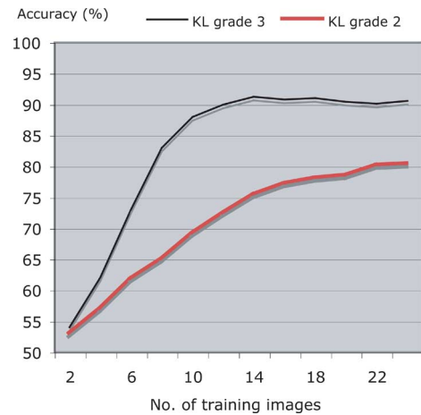
Fig. 4. Classification accuracy (%) of KL grades 2 and 3 as a function of the size of the training set.
