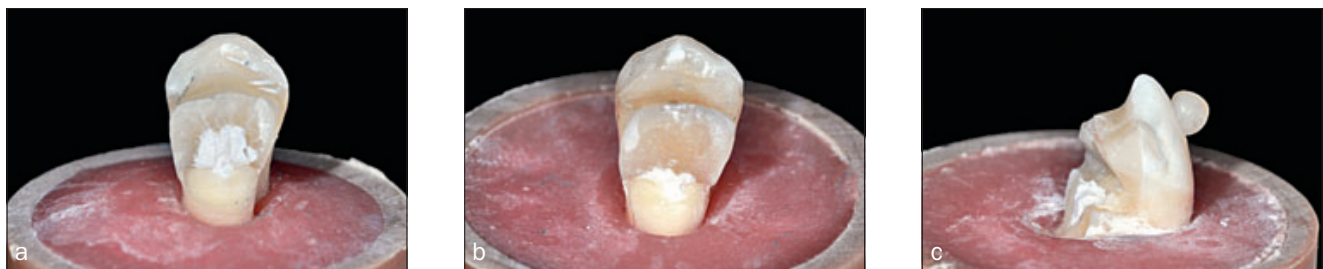
Fig 3 Fracture modes observed in the study: a – type I fracture occurring in the RelyX ARC group: cusp fracture at the CEJ; the fracture was in the tooth/inlay interface, preserving the restoration; b – type II fracture occurring in the RelyX Unicem group: cusp fracture below the CEJ; the fracture was in the tooth/inlay interface, preserving the restoration; c – type IV fracture occurring in the RelyX ARC group: cusp fracture below the CEJ; the fracture was in the composite resin inlay first, preserving the tooth/inlay interface and leaving part of the restoration attached to the cusp.
