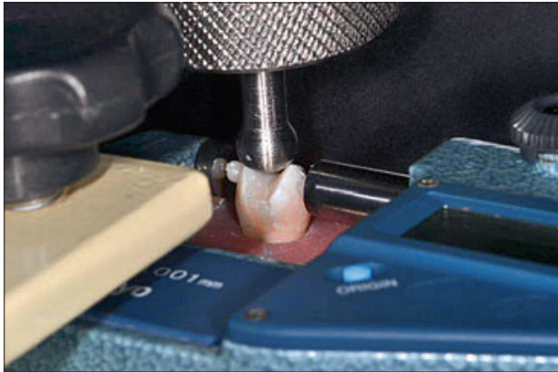
Fig 2 Cuspal deflection test: the resin spheres are positioned on the cuspal vertices and served as reference points for measuring the intercusp distance using a micrometer. A steel sphere with 8-mm diameter contacts the buccal and palatal cuspal inclines.
