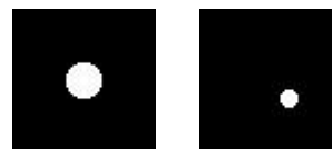
Fig. 2. Geometrical Models. On the left, cylinder filled with water and activity of 50 \mu\text{Ci}/\text{cm}^3 . On the left, punctual source filled with water and activity of 30 \mu\text{Ci}/\text{cm}^3 (not centered).
