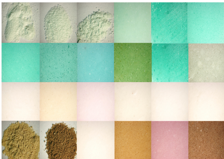
Fig. 15. Examples of synthetic talc colors by partial or complete substitution of magnesium by others divalent cations.
