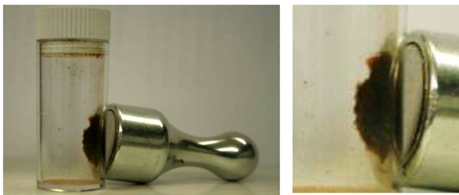
Fig. 18. Magnetic synthetic talc attracted by the magnet. Note that all the powder is attracted to the magnet.
