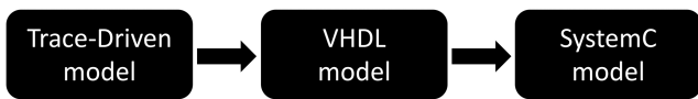
Fig. 4 Different abstraction layers are necessary to cover evaluations with distinct goals, ranging from accurate to fast simulations
