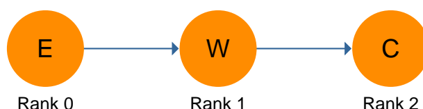
Figure 5.5 – Early MPI DSPARLIB layout proposal, single Worker.
