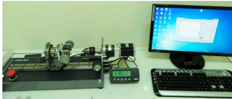
Figure 7. Image of the torque machine used for the torque removal measurements.
