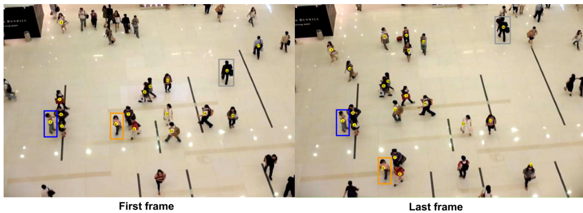
(a) Start and end of Video A, highlighting pedestrian 2 (blue), pedestrian 6 (orange) and pedestrian 16 (gray)
