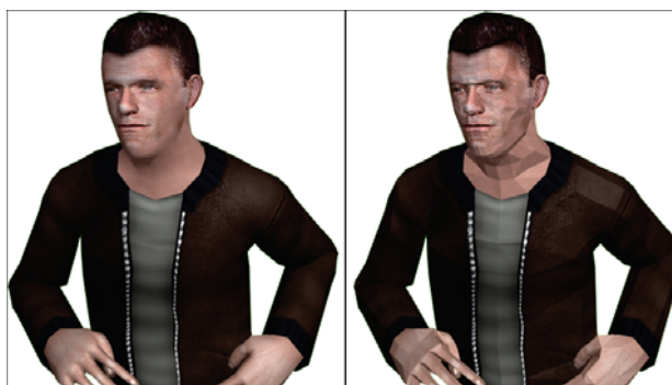
Figure 4.4 – Illustration of a virtual human using normal map technique (left) and using regular lighting technique (right).
