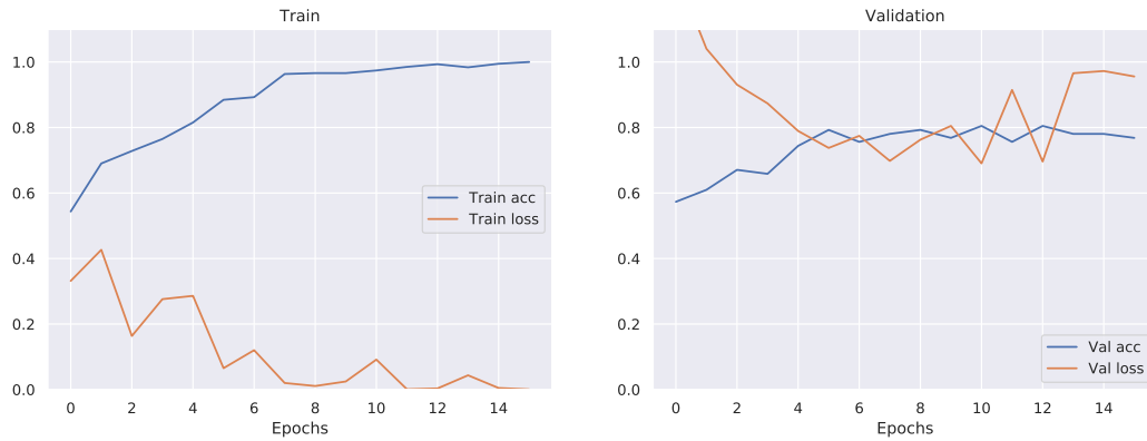
Figure 3.4 – Progress of the loss and the accuracy of the NCC-Model throughout the training steps using the hyperparameter values of Table 3.5
