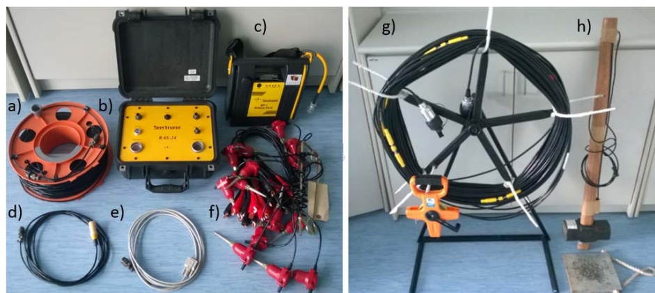
Figure 1. a) Extension of the trigger, b) RAS-24, c) 12v battery, d) trigger e) serial cable, f) 12 geophones, g) connection cable of 120m for the geophones, h) 8kg hammer and aluminum plate 20x20 cm.
