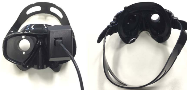
Fig. 4. Experimental Equipment. During tests, a camera is fixed to one of the eyes, while the other opening is kept closed.
