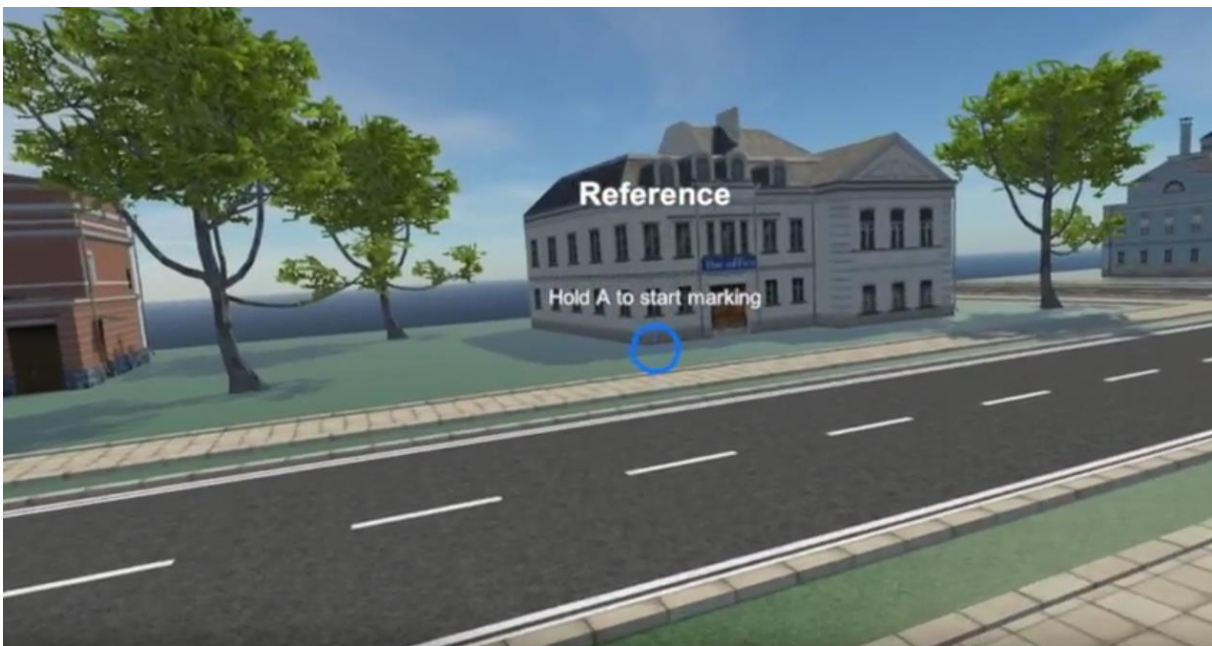
Figure 27 - Simulated augmented reality environment. Digital models were used to create a small town, and the geometry was unknown to the application. The interface elements include the tool's name, the tool's tip on usage, and a blue cross-hair, which defines the point of interaction.
