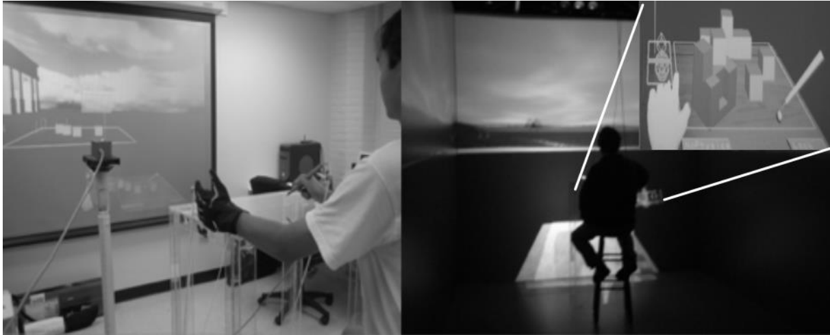
Figure 12 - Massing study environment using a projector (left) and a CAVE (right)
