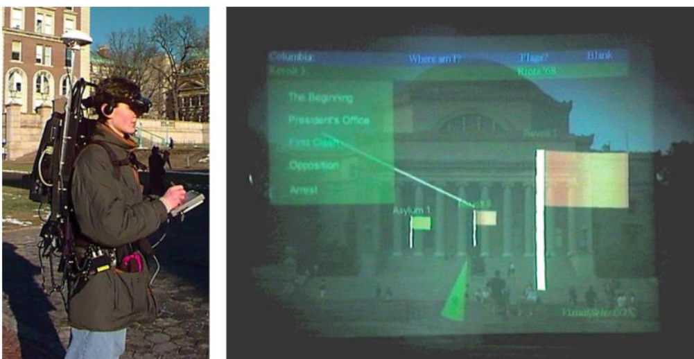
Figure 9 - A Touring Machine: backpack (left); the head-worn display showed information about buildings and landmarks (right)
