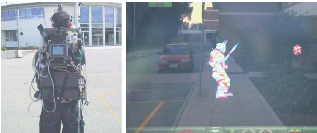
Figure 10 - ARQuake application. The tinmith system (left) was used to recreate the classic game Quake in augmented reality. The displayed showed the game overlaid to the real world (right).
