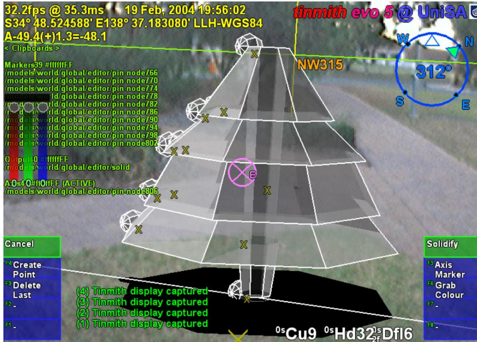
Figure 22 – Surface of revolution technique allows the creation of volumes with radial symmetry.
