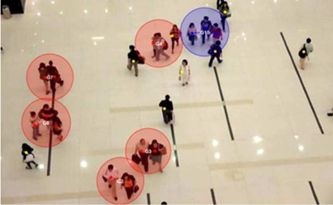
Figure 4.5: Group detection example : six groups detected, being five permanent, in red, and one temporary, in blue.
