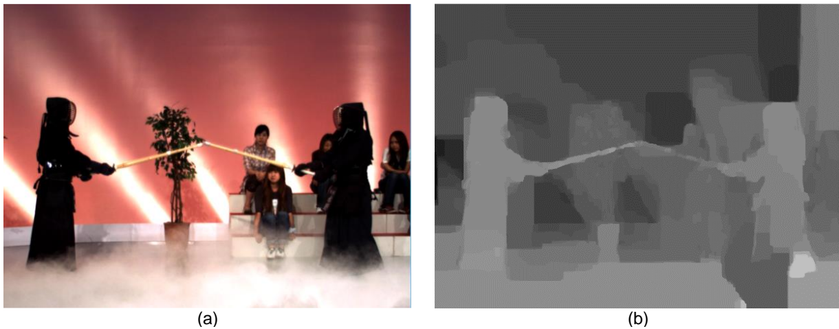
Figure 1.1 – (a) Texture view and its associated (b) depth map obtained from Kendo video sequence (source: [75]).
