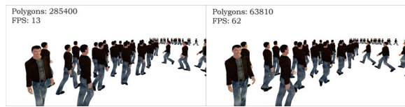
Figure 13: Illustration of the exact same scene and camera view for 100 agents in two different renderings without any LOD technique (left) and with LODs technique and impostors (right).
