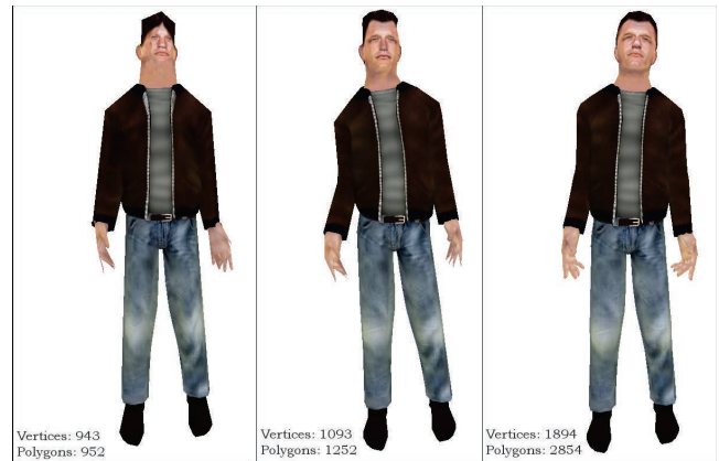
Figure 7: Illustration of one virtual human and the three Levels-Of-Detail, low quality (left) medium quality (center) and high quality (right), with the respective number of triangle and polygons.
