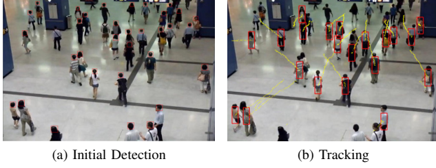
Fig. 2. Tracking phase in our approach: (a) the input image and heads detection, and (b) the people detection and tracked trajectories.
