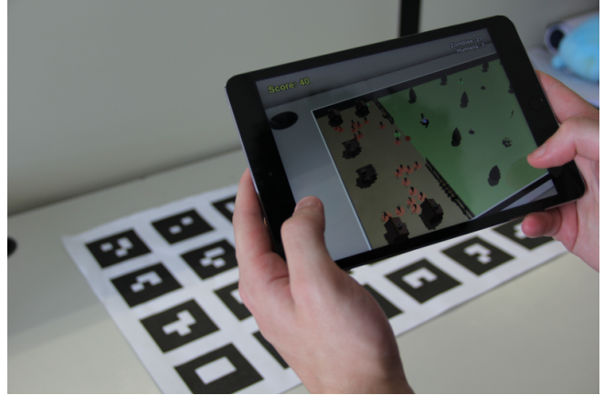
Figure 3. User playing. User points to the markers and the environment is rendered
