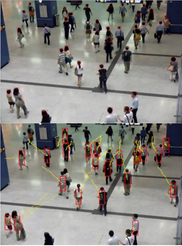
Fig. 1. The group features are obtained applying the approach presented by Favaretto et al [22]. On the top: the input image and heads detection, and on the bottom: the people detection and tracked trajectories.
