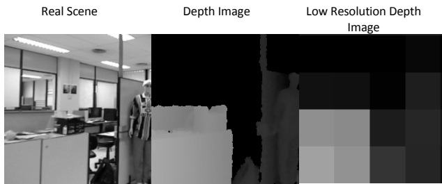
Figure 3 – Depth map downsampling process
