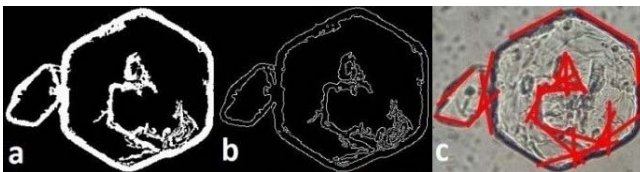
Figure 5: Blob identified (a), blob processed by the Canny algorithm (b), lines detected by the Hough transform (c)
