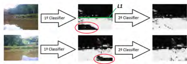
Figure 5: On the left are the two input images; the images of the middle show the results from the classification of the first ANN, with reflection zones marked by the ellipses; the images on the right side show the result with the combination of both ANN classifiers.
