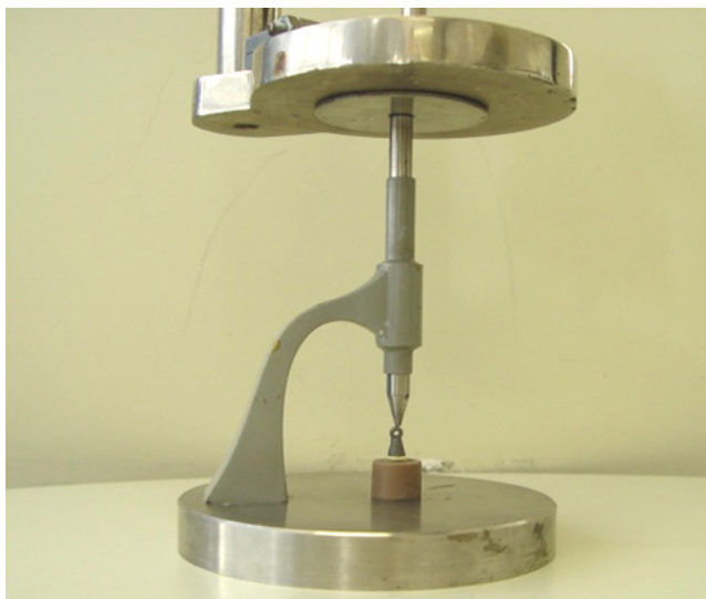
Figure 2. Specimen fabrication. Each metallic coping was luted on the abutment under an axial force of 5 kg for 10 min.
