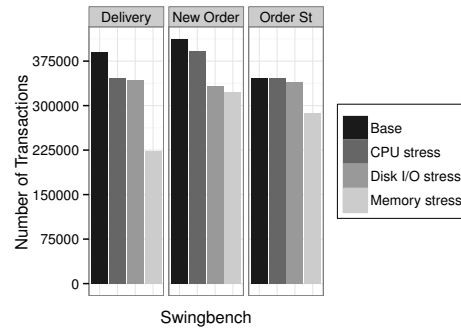
Fig. 4. Performance interferences in the database transactions on LXC with CGroups
