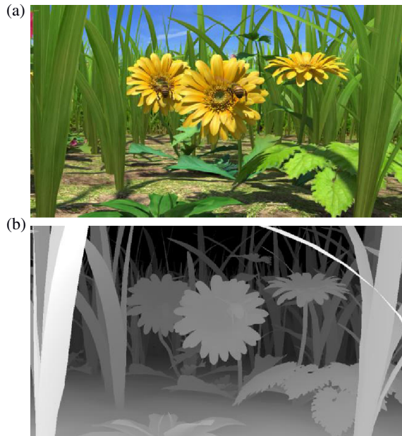
Fig. 1 (a) Texture view and its associated (b) depth map extracted from MicroWorld video sequence. 7
