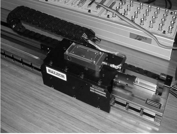
Fig. 1. Experimental set up of the electromagnetic motor.
