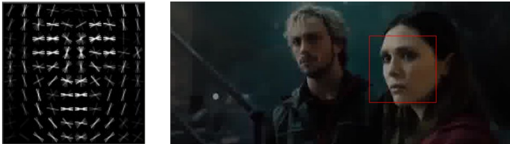
Figure 3.8: On the left, the gradients orientation of HOG face detection descriptor. It is important to notice that the gradients directions result in a face shape, which helps to understand the intuition behind HOG and why it works. On the right, the face identified by the given descriptor.
