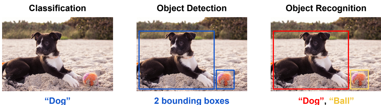
Figure 2.13: Comparison between image classification, object detection, and object recognition.
