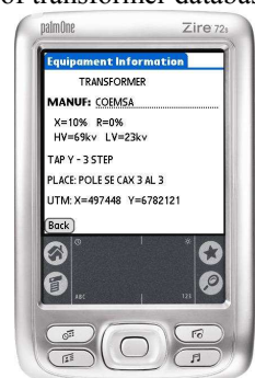
Figure 11 - Results of transformer database query.
