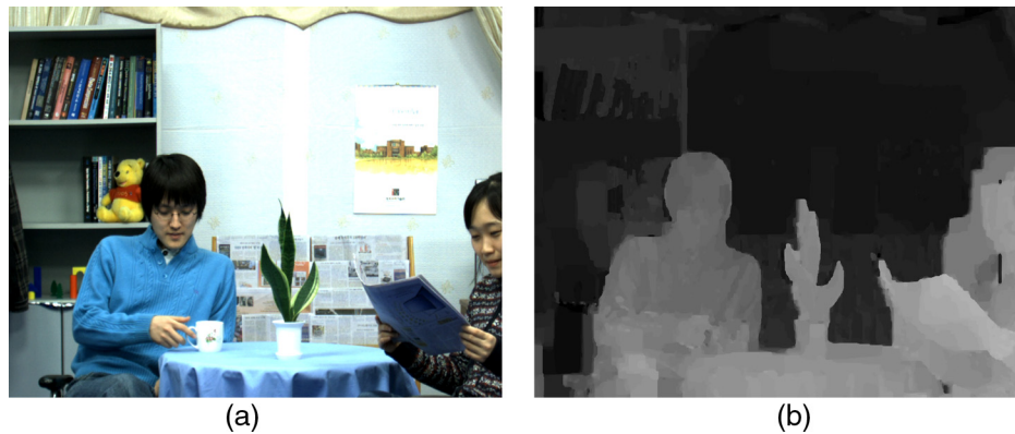
Fig. 1 (a) Texture view of the first frame of Newspaper_CC video and its associated (b) depth map.
